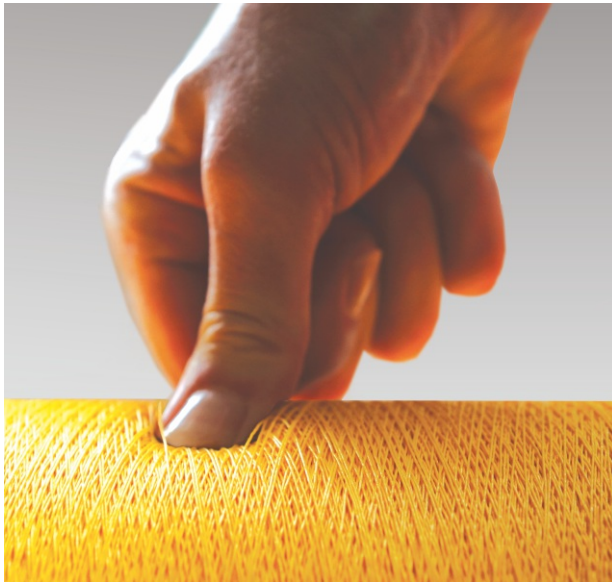
Fewer cross marks due to soft bobbins
